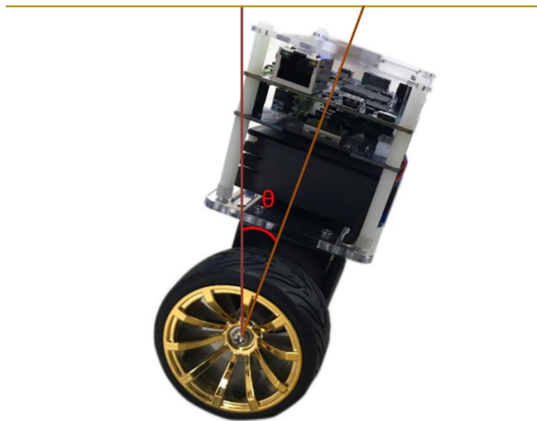
Figure 1- 10 The tilted angle of the balance car
