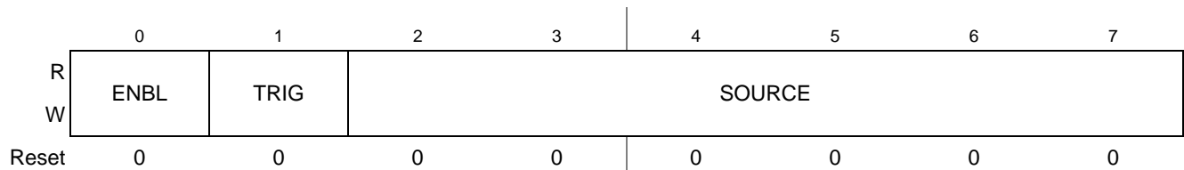
Figure 13-2. Channel Configuration Registers (CHCONFIG n )
