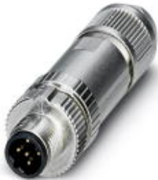
Bus system connector, male, straight, 2-pos., M12 SPEEDCON, shielded, B-coded, spring-cage connection, metal knurl, cable cross section max. 8 mm
