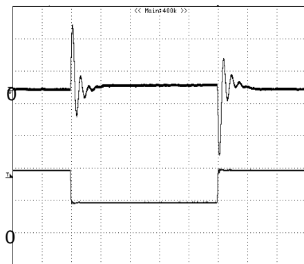
Figure 9: Output voltage response to step-change in load current (75%-50%-75% of I_{o, max} ; di/dt = 1.0A/\mu s ). Load cap: 100 \mu F tantalum capacitor and 1 \mu F ceramic capacitor. Top Trace: V_{out} (100mV/div, 200 \mu s /div), Bottom Trace: I_{out} (10A/div). Scope measurement should be made using a BNC cable (length shorter than 20 inches). Position the load between 51 mm to 76 mm (2 inches to 3 inches) from the module
