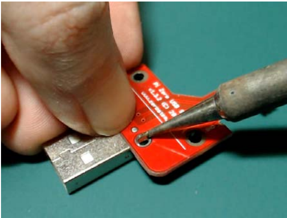
7. To align the connector, reflow the solder on the tab joint while pressing down on the Zero Stem PCB.
