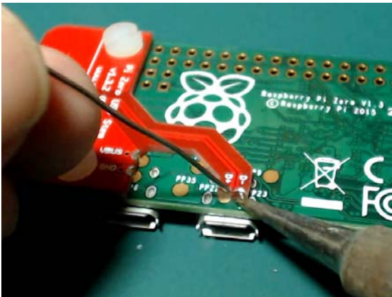
15. Solder the four Zero Stem castellations to the Pi Zero test points.
