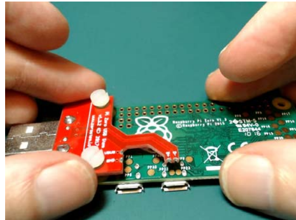
12. Align the Zero Stem PCB bolts with the mounting holes in the Pi Zero.
