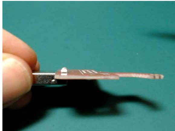
8. Check the connector is aligned correctly. It should be flush with the Zero Stem PCB.
