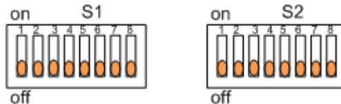
Figure 13: S1 and S2 configuration for external application control through USB
