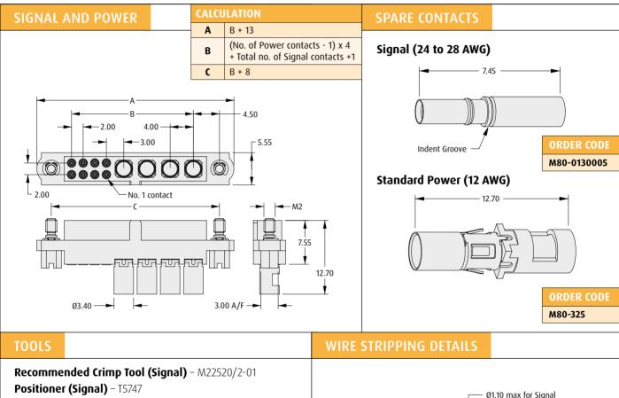
Contact Insertion/Removal Tool (Signal) - Z80-280 Contact Removal Tool (Power) - Z80-290
