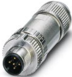
Bus system connector, connector, straight, 5-pos., M12 SPEEDCON, shielded, A-coded, spring-cage connection, metal knurl, cable diameter max. 8 mm
