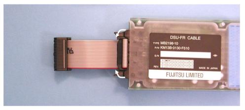
The DSU cable is now ready to be connected to the MB2198-100 Adapter Board. Therefore plug in the ribbon cable to the socket with the two lock levers.
