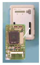
Mount the Adapter Board MB2198-210 to the Emulator Main Unit MB2198-01. Be sure that the two small white triangles of the connectors point together.
