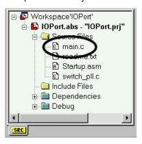
The left window shows the Structure of the work space including the source codes, include files, header files and debugger information.
