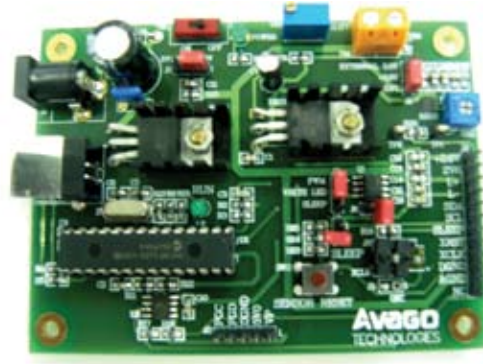
Figure 2. Digital Color Sensor Controller Board
