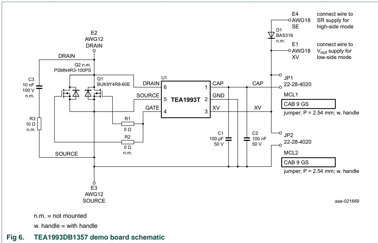
[Figure 6](#) shows the schematic diagram of the TEA1993DB1357 demo board. The board incorporates the TEA1993TS SR controller and a power MOSFET. The TEA1993TS acts as a controlled amplifier. The input is the voltage difference between the DRAIN and the SOURCE pin. The corresponding gate driver signal is the output. The amplifier regulates the source-to-drain voltage difference to 35 mV in the rectification phase.
