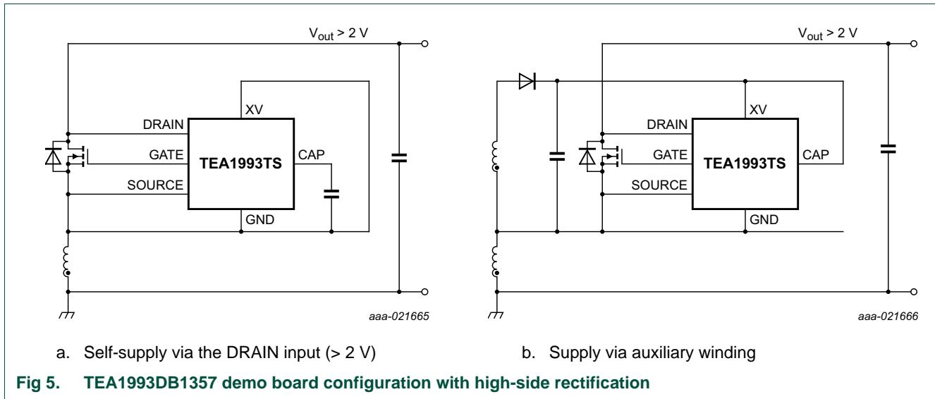
**Fig 5. TEA1993DB1357 demo board configuration with high-side rectification**
