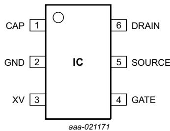
Fig 3. Pin configuration TEA1993TS (TSOP6)
