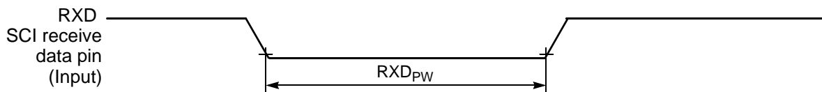
Figure 10-16 RXD Pulse Width
