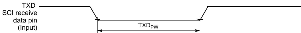
Figure 10-17 TXD Pulse Width
