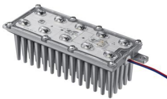
(a) Module with Fin [Thermal management by Module/Engine]
