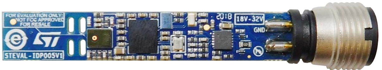
Figure 4. STEVAL-IDP005V1 board - bottom
