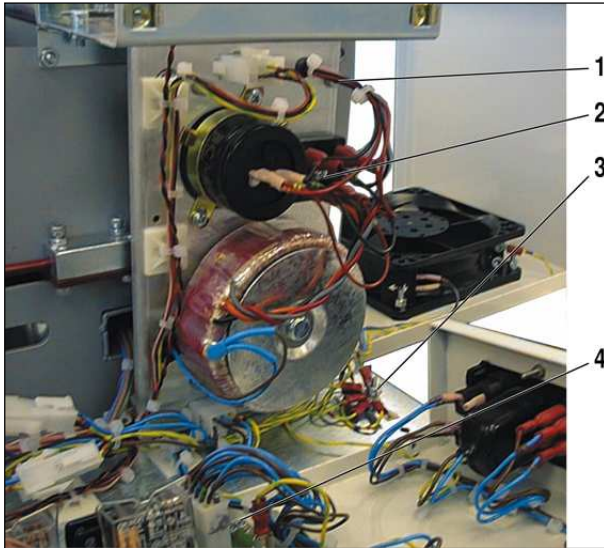
Fig. 4-18: 24V DC PSU Location
