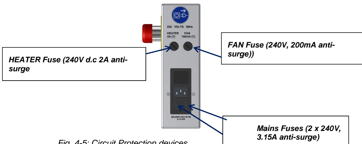
Fig. 4-5: Circuit Protection devices
