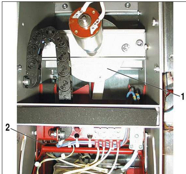
Fig. 4-11: Motor Disk Assembly
