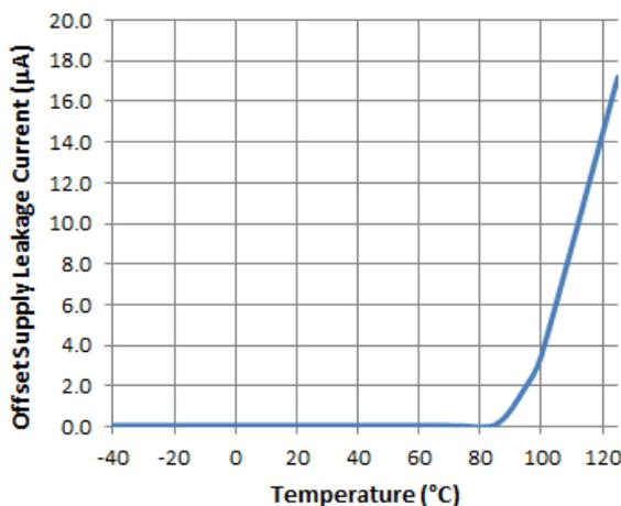
**Figure 26.** Offset Supply Leakage Current vs. Temperature
