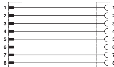
Contact assignment of the M12 plug and the M12 socket
