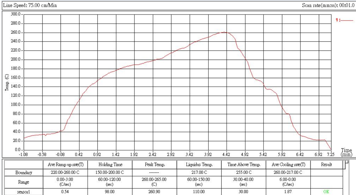
Figure 8.5 Solder Reflow Profile
