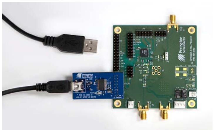
Figure 4. PLL USB Interface Board Connected to the PE33241 Evaluation Board for Serial Programming
