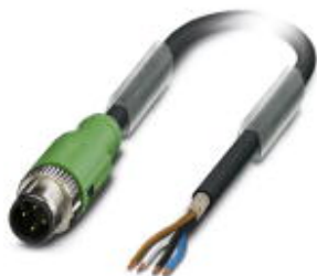
Sensor/actuator cable, 4-position halogen-free, black-gray RAL 7021, shielded, Plug straight M12 SPEEDCON, A-coded, on free cable end, cable length: 5 m
