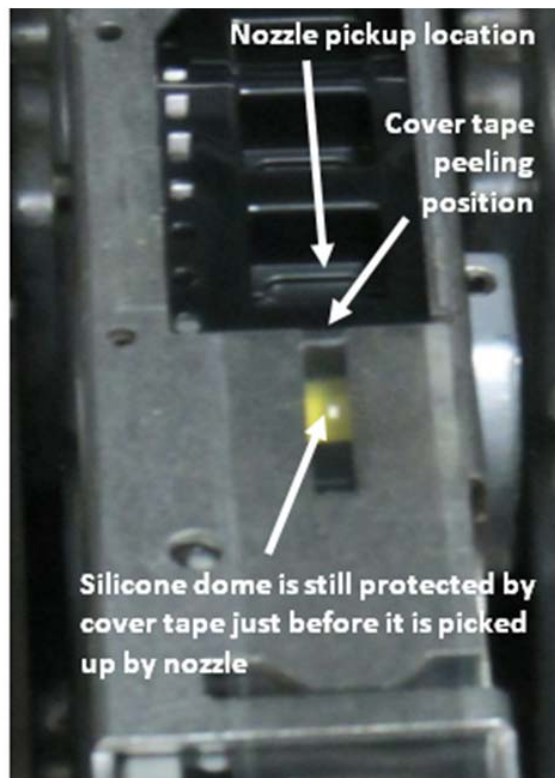
Figure 15. Example of a modified feeder which protects the silicone dome prior to pickup.
