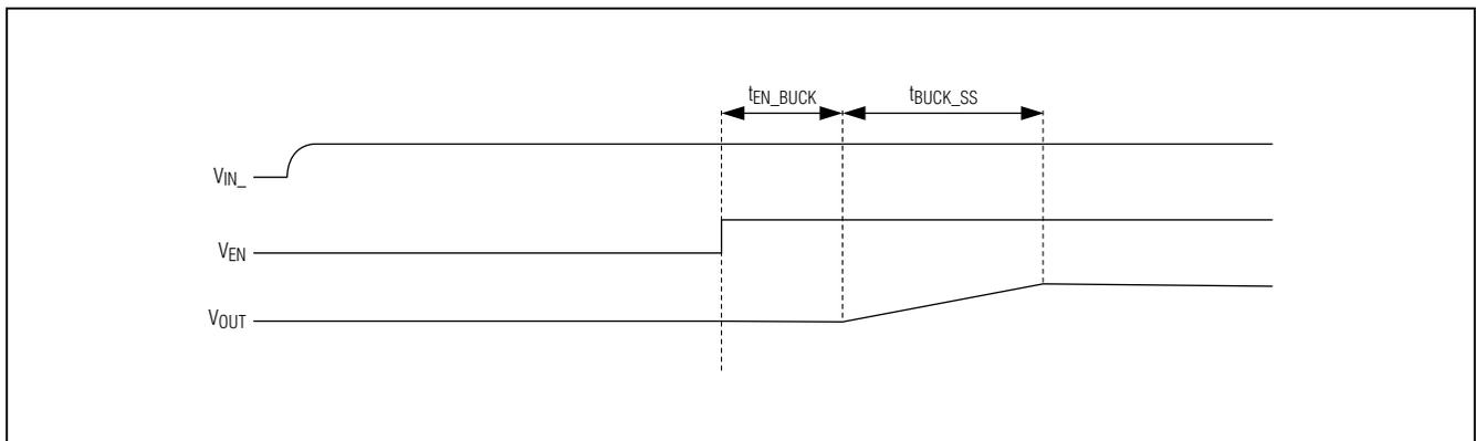
Figure 2. Power-Up Timing
