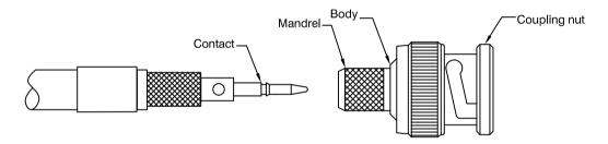
3) Insert the contact into the body and ensure that the contact captivates. Make sure that the braid is on the outside of the mandrel. Slide the ferrule over the braid until the ferrule butts up against the body. Crimp the ferrule using the correct tool for the connector.
