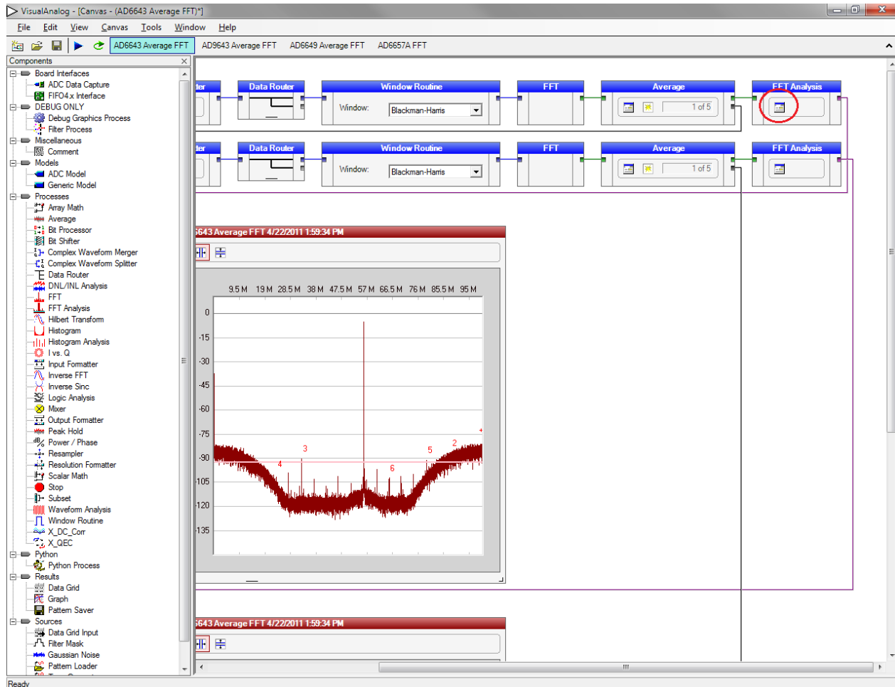
Figure 20. VisualAnalog, Main Window—Showing FFT Analysis for AD6643
