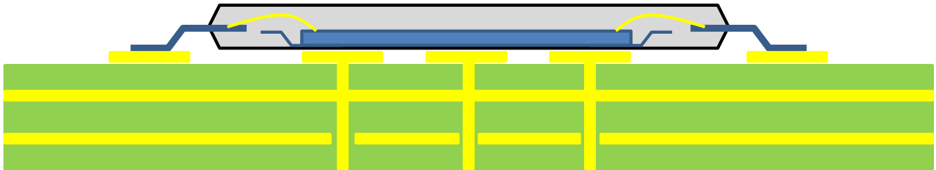
Figure 10.2-1: Example thermal via holes on PCB.
