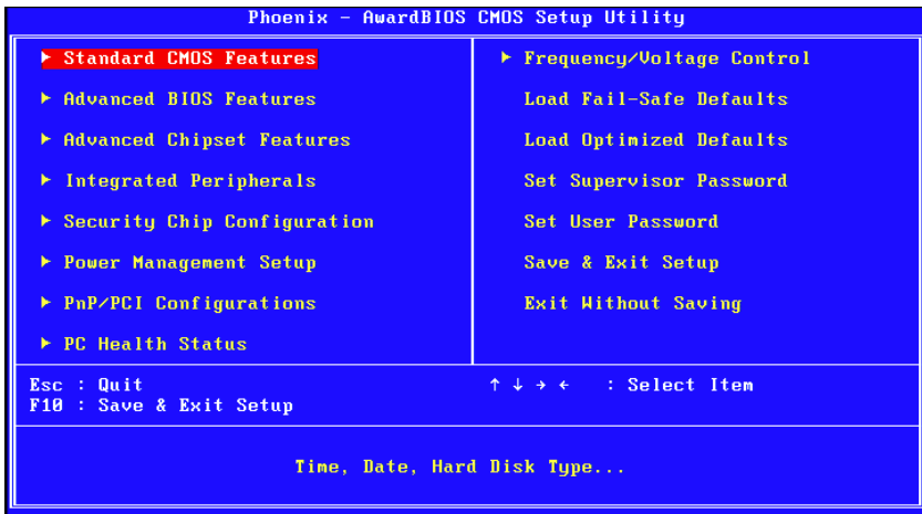
Figure 2.1: Award BIOS Setup initial screen
