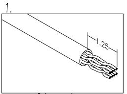
REMOVE 1.25" (31.8 mm) OF CABLE JACKET AND UNTWIST WIRE PAIRS.
