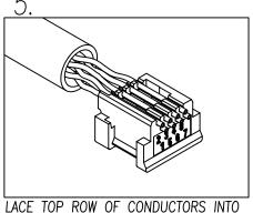
LACE TOP ROW OF CONDUCTORS INTO LOADBAR. TRIM TOP ROW OF CONDUCTORS FLUSH.
