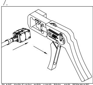
PLACE CABLEJACK INTO HAND TOOL AND TERMINATE.
