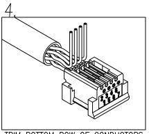
TRIM BOTTOM ROW OF CONDUCTORS FLUSH WITH LOADBAR.
