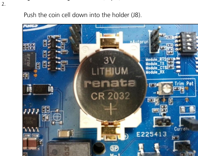
Figure 15: Inserting the coin cell (step 2)
