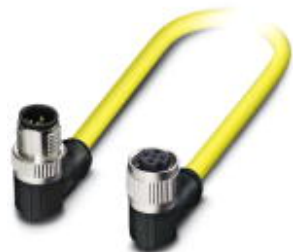
Sensor/actuator cable, 5-position, PVC, yellow, Plug angled M12 SPEEDCON, A-coded, on Socket angled M12 SPEEDCON, A-coded, cable length: 5 m
