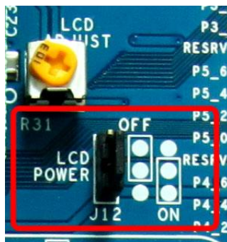
Figure 4-4: CY8CKIT-001 PSoC DVK LCD Power Jumper
