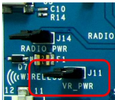
Figure 4-5: CY8CKIT-001 PSoC DVK VR_POWER Jumper
