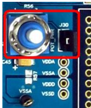
Figure 4-7: CY8CKIT-030 PSoC 3 DVK Potentiometer Power
