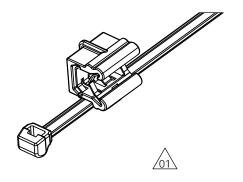
**DELIVERY CONDITION:** CABLE TIE HEAD COULD BE AT THE LEFT OR RIGHT SIDE OF EDGE CLIP
