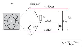
All voltages measured to ground External load resistor  ${\rm R}_a$  from  ${\rm U}_A$  to  ${\rm U}_{BA}$  required.
