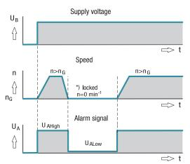
\* Speed limit  $n_G = 0 \text{ rpm}$
