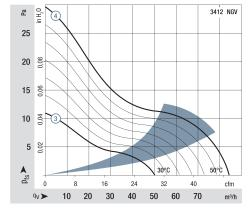
Air performance measured according to: ISO 5801. Installation category A, without contact protection. Noise: Total sound power level  $L_{W}A$  ISO 103002 measured on a hemisphere with a radius of 2 m. Sound pressure level  $L_{p}A$  measured at 1 m distance from fan axis.
