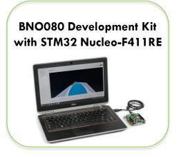
Co-developed by Hillcrest Labs and Bosch Sensortec, the BNO080 is a single chip solution that integrates an accelerometer, a gyroscope, a magnetometer, and a low-power 32-bit ARM Cortex M0+ MCU, running Hillcrest's high-performance sensor hub software stack.
