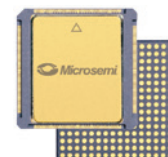
b.s. 0.67" x 0.67" (17 mm x 17 mm) h. 72 mils (1.847 mm) p. 7.5 mils (0.19 mm)
