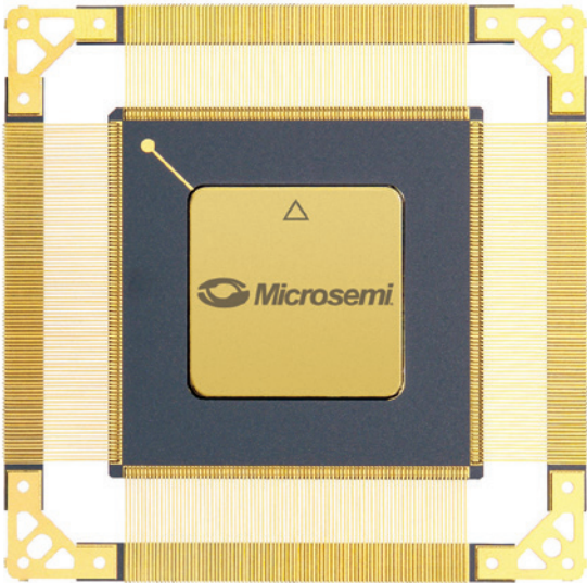
CQ352 b.s. 1.890" x 1.890" (48 mm x 48 mm) h. RTAX—105 mils (2.67 mm) h. RTG4—89 mils (2.25 mm) p. 20 mils (0.50 mm)
