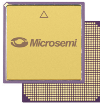
RTAX4000S, RTAX4000SL, and RTAX2000D only b.s. 1.457" x 1.457" (37 mm x 37 mm) h. CCGA—218 mils (5.535 mm) h. CLGA—129 mils (3.28 mm) p. 39 mils (1.00 mm)
