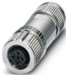
Bus system connector, female, straight, 2-pos., M12 SPEEDCON, shielded, B-coded, spring-cage connection, metal knurl, cable cross section max. 8 mm
