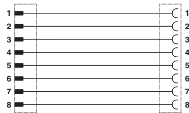
Contact assignment of M12 connector/socket
