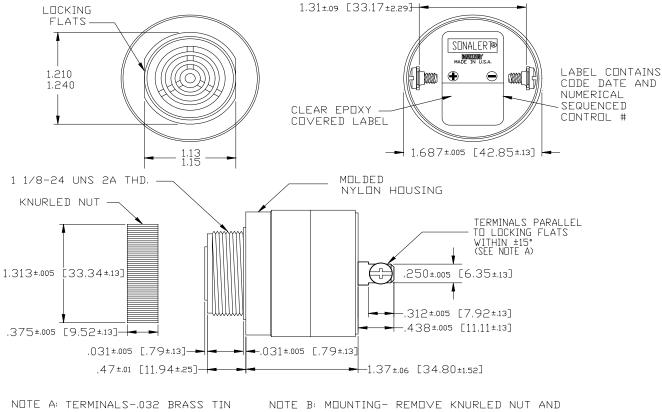
NOTE A: TERMINALS-.032 BRASS TIN PLATED, TAPPED FOR #6-32 SCREW. TWO #6-32 NICKEL PLATED BRASS SCREWS INCLUDED. WILL ACCEPT 1/4" QUICK CONNECT. NOTE B: MOUNTING- REMOVE KNURLED NUT AND
