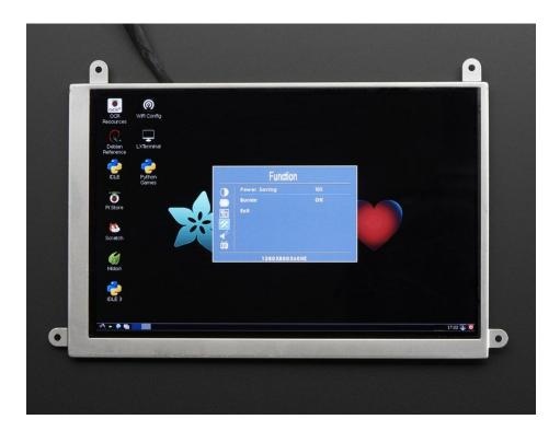
$\label{lem:section} \textbf{Power Saving - 10s to 60s - how long it takes for the screen to shut off} \\ \textbf{Burnin - On/Off - a function to prevent screen burn-in (https://adafru.it/dTR)}$
