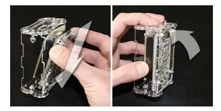
Now tip the face plate in the opposite direction and install the case top in a similar fashion. Align the hole in the top face with the reset button on the BeagleBone (once sealed, this is accessed with a paper clip or small screwdriver). Or you can choose to keep the top cover off, if you'll need frequent access to the BeagleBone or cape.
