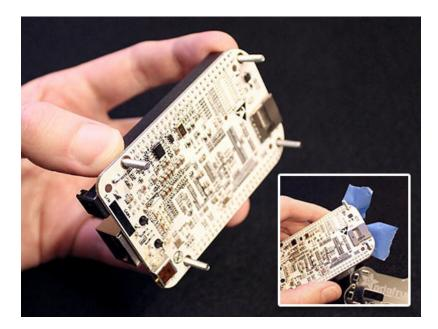
Slide a nylon spacer over each of the four screws. VERY IMPORTANT: Use ONLY the spacers included with the kit. DO NOT use wider standoffs or spacers in their place, and SUPER ESPECIALLY DO NOT use hex-nuts as a makeshift standoff/spacer. The component clearances on the BeagleBone are *very* close, and using the wrong spacers could result in components being crushed!
