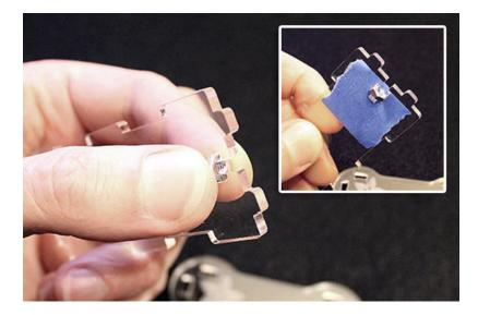
Position one of the end pieces over the alignment studs, then insert a screw through the corresponding hole for the nut. Tighten with gentle finger pressure for now.
