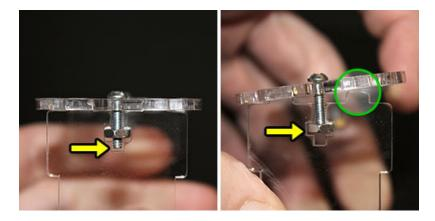
Insert the BeagleBone base plate into the case by inserting the alignment studs into the back face, then pivot the
