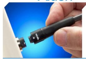
Ideal for rear-panel instrumentation and hand-held equipment, the compact and cost effective PL-500SM-N Series is designed to meet the efficient packaging demands of portable electronic devices
