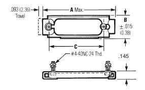
Consists of Lock Retainer and two lock posts (order separately). NOTE: Not compatible with D\*H Series or SDH Series backshells.
