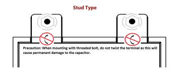
Hardware: M6≈1/4-20 stud / bolt Copper flat washer, M6 washer with 12 mm (0.472") OD
