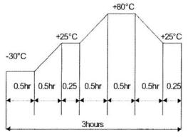
The diaphragm will be measured after being placed at +25°C for 4 hours. The value of the resonant frequency should be  $\pm 10\%$ , the value of the electro static capacitance should be  $\pm 20\%$  compared to the initial measurements. The resonant impedance should be 2,000  $\Omega$  max.
