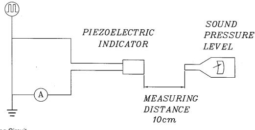
S.P.L. Measuring Circuit Input Signal: 10 Vp-p, 5.0 KHz, square wave Mic: RION S.P.L. meter UC30 or equivalent S.G.: Hewlett Packard 33120A function generator or equivalent
