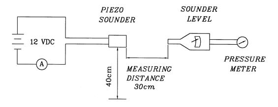
S.P.L. Measuring Circuit Mic: RION S.P.L. meter UC30 or equivalent
