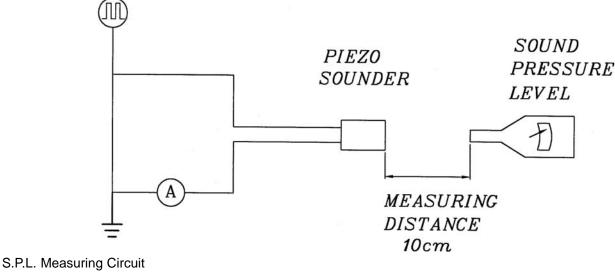
Input Signal: 10 Vp-p, 4.0 KHz, square wave Mic: RION S.P.L. meter UC30 or equivalent
