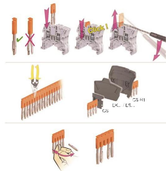
Additional accessories must be installed on the cut side of the jumper bar with cut extremities:
