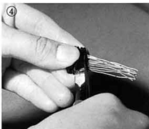
4. Cut the extra cable length extended from the holder with nipper or cutter.
