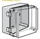
Includes two polyamid hinges, eight M4 self-tapping zinc-plated screws, eight flat washers and drilling template. Use on all QLINETM E enclosures. Kit might not meet Type 4 requirements and should, therefore, be verified by customer.
