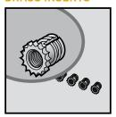
Self-tapping Brass Inserts fit into molded pads in the bottom of the enclosure. Inserts have an M2 internal machine screw thread and M4 self-tapping external thread.
