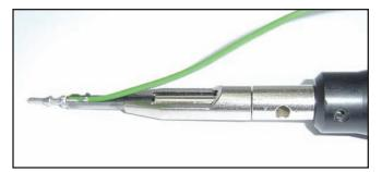
Insert contact into the connector until it snaps in by applying constant pressure. Note: Make sure that the contact and tool are inserted parallel to the insulator axis. Do not tilt!
